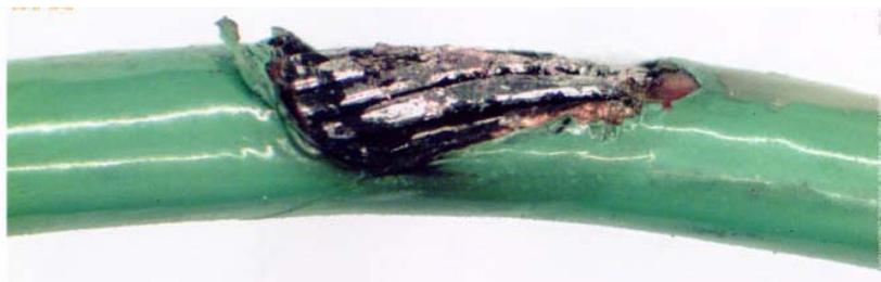
Figure 2: Damaged wire that resulted from a short to ground on the space shuttle.
