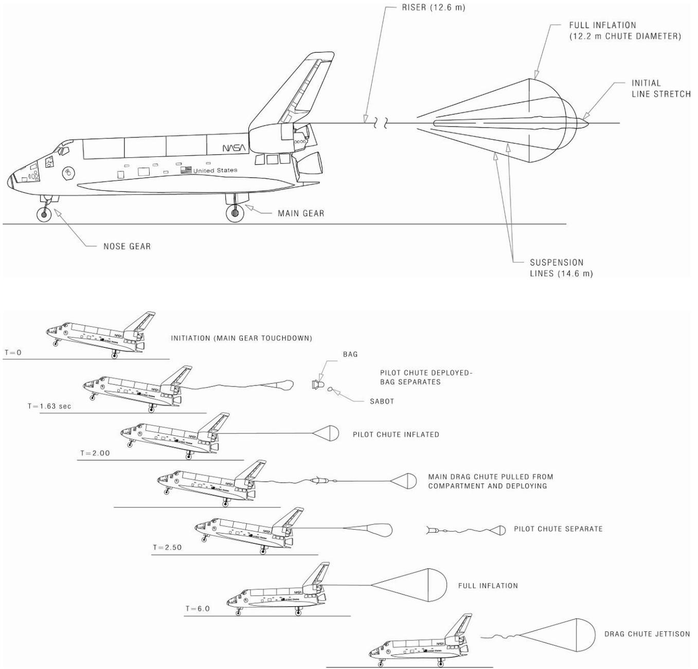
Figure 2: Space shuttle main gear touchdown through chute jettison.
