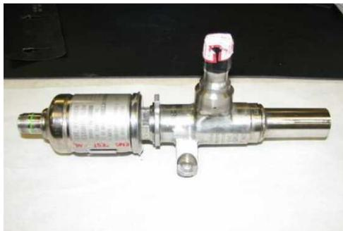
For the shuttle engines to run correctly and for the hydrogen tank to maintain structural integrity, the LH2 tank pressure is regulated to 33 psi. For single flow control valve failures, the other two valves can compensate by moving to either the high or low flow position as required. In some cases, the other valves can not compensate and the tank pressure can reach 35 psi. In this event, a vent valve on the tank can open to relieve the pressure.
