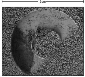
While the Viking and Mars Pathfinder landers could not measure soil consistency, the Mars Exploration Rovers pressed the RAT (Rock Abrasion Tool) into the martian soil and photographed the impression. By studying how well the soil held together, scientists gathered valuable data on soil consistency. Scientists also used the rovers' wheels to dig trenches and compact the soil.
