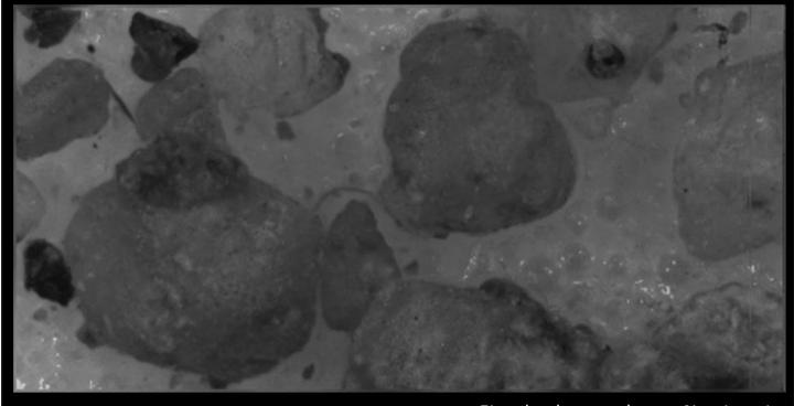
Phoenix microscope image of beach sand, the largest grains are  $500 \ \mu m$  in diameter.
