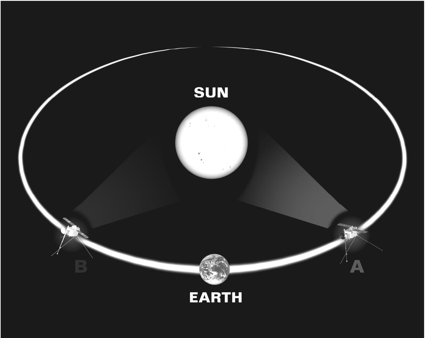
The STEREO observatories will orbit the Sun in a heliocentric orbit at ~1 Astronomical Unit (AU), with one leading Earth and one lagging.
