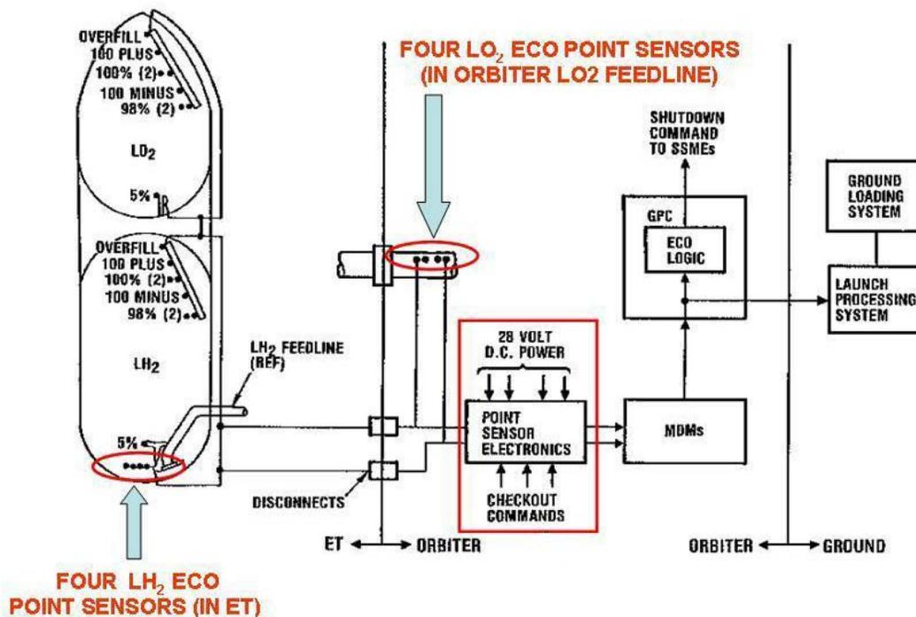
**Figure 6.0-1. ECO and Liquid Level Sensors Block Diagram**
