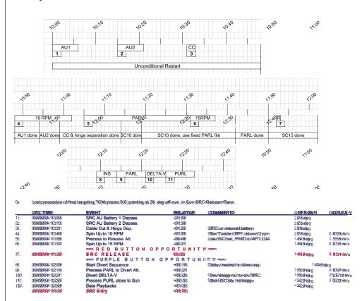
The final decision (Purple button) was the command to enable the spacecraft to execute the same divert maneuver to put the spacecraft en route to a safe disposal orbit. If the SRC did not separate from the spacecraft (i.e., if the cable had not fully cut and the two bodies were dangling with a soft connection), this final decision would cover the contingency. The final decision timeline is shown in Figure B-8.
