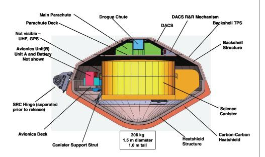
Figure B-4. SRC cross section (SRC hinge is separated from SRC prior to release).
