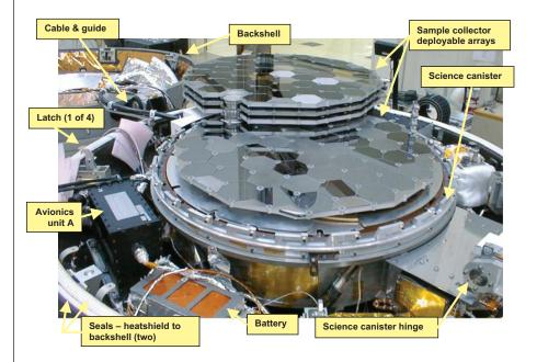
*Eigure B-6. SRC prior to installing thermal closures – avionics box A and the LiSO, battery in foreground.*  Temperature strips were attached to the inside honeycomb structure of the heatshield and backshell to record the maximum temperature reached during entry and heat soak back.
