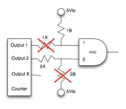
Figure 7.1. Example of EST timing circuit and timing jumper/ resistor placements. During the inspection of the EST board from avionics box B, all the resistors were determined to be installed in the proper configuration to achieve the stated signal timing.
