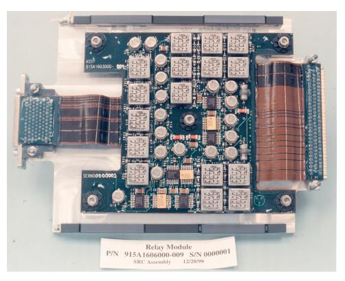
Figure 4.2. Relay card close-out photograph.
