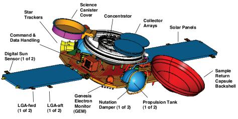
\* Genesis Ion Monitor (GIM) is caddy corner GEM, on +Xsv deck (fwd) \* MGA and thrusters on -Xsv deck, towards -Xsv-axis (aft) *Figure B-2a. Spacecraft in science collection configuration, sun view.*
