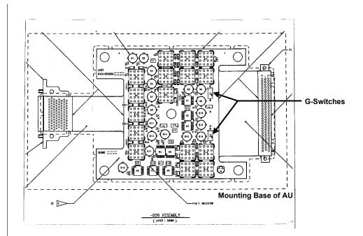
Figure 4.1. Relay card assembly drawing.
