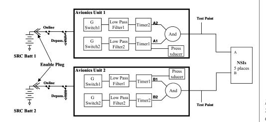
Figure 1.9. SRC pyrotechnic firing circuit layout.
