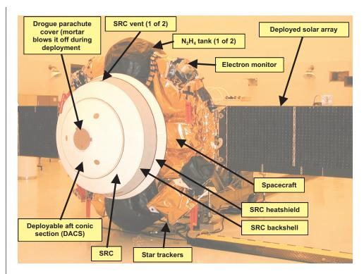
Figure 1.5. Flight configuration with thermal blankets installed.
