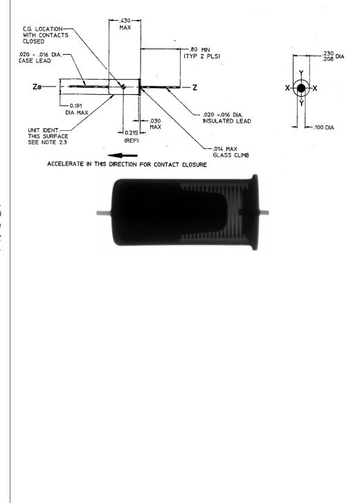
Figure B-14. Aerodyne 7200-6-000 acceleration switch (G-switch sensor) drawing and X-ray.
