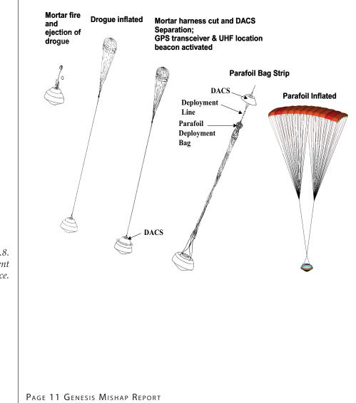
Figure 1.8. Parafoil deployment sequence.
