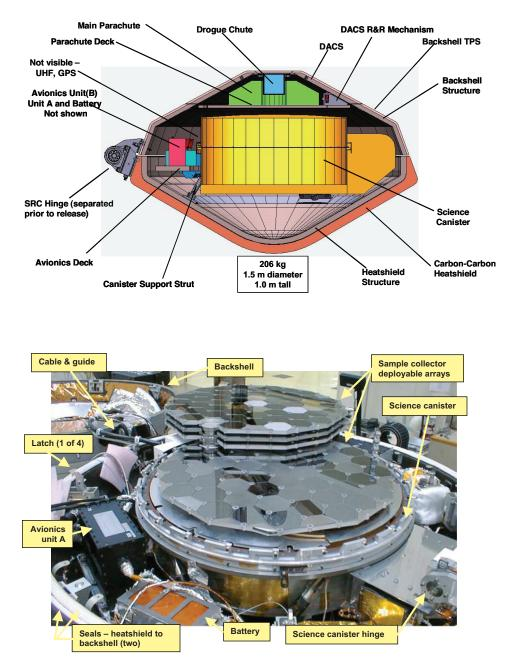
Figure 1.6. SRC cross section (SRC hinge is separated from SRC prior to release).
