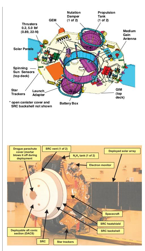
Figure B-2b. Spacecraft in science collection configuration, anti-sun view.
