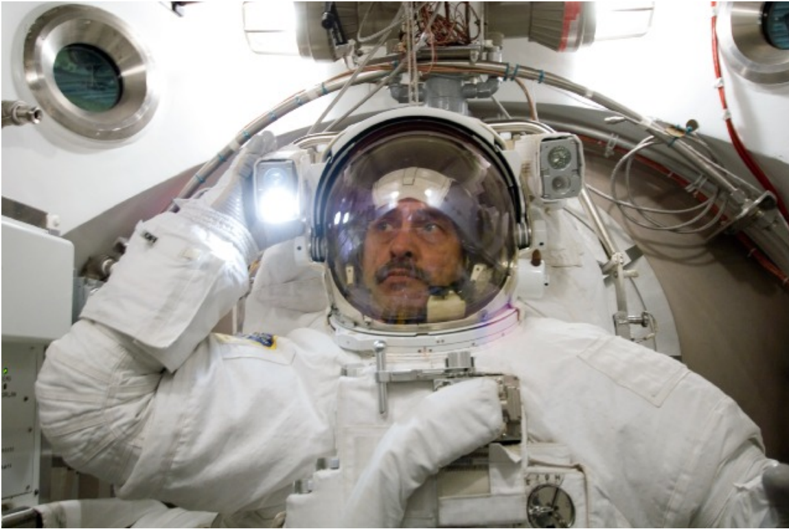
Cosmonaut Pavel V. Vinogradov, Expedition 13 commander representing the Russian Federal Space Agency, participates in an Extravehicular Mobility Unit (EMU) spacesuit fit check in the Space Station Airlock Test Article (SSATA) in the Crew Systems Laboratory at the Johnson Space Center.
