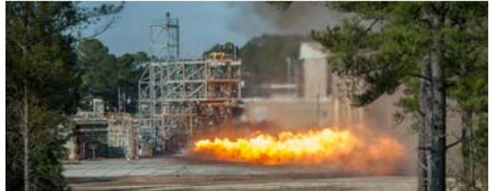
*The gas generator from an F-1 engine is test-fired at the Marshall Space Flight Center in Huntsville, Ala., on Jan. 24, 2013. Data from the 30 second test will be used in the development of advanced boosters for NASA's Space Launch System, which is managed at the Marshall Center.*
