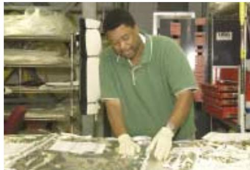
A technician checks an orbiter Thermal Control System Blanket that will be used on a future flight.
