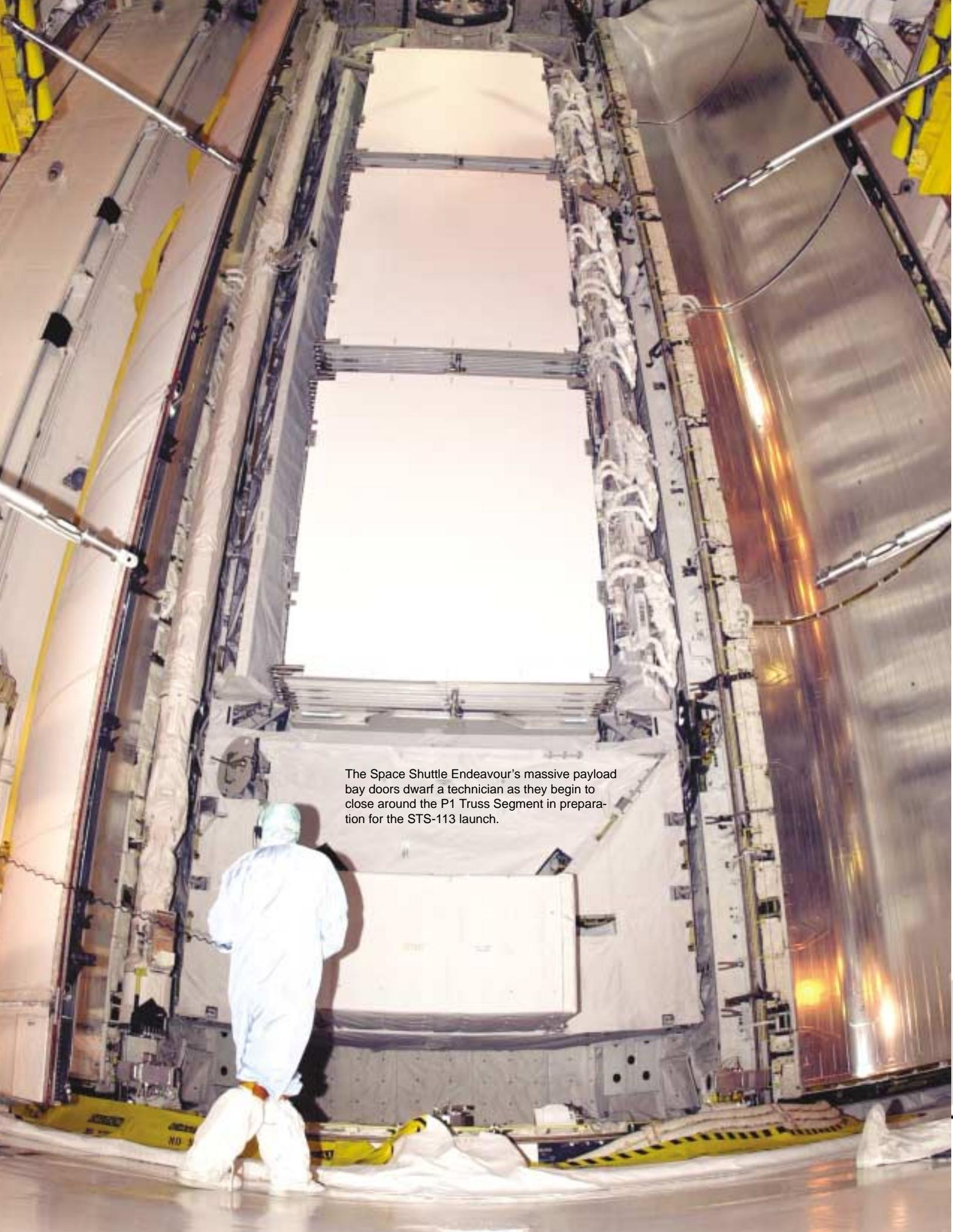
The Space Shuttle Endeavour's massive payload bay doors dwarf a technician as they begin to close around the P1 Truss Segment in preparation for the STS-113 launch.
