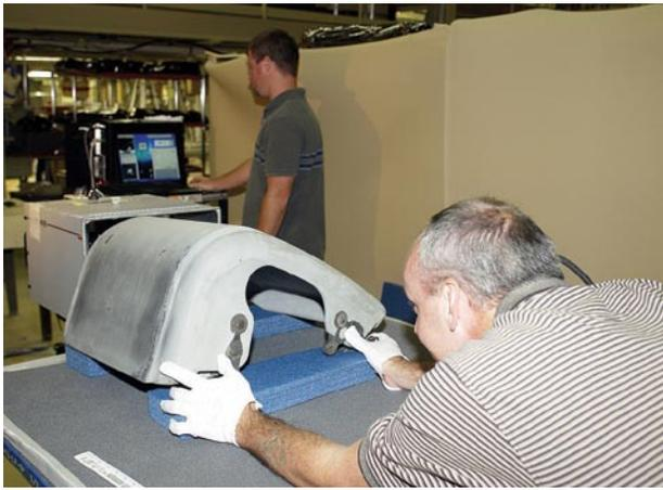
In the Orbiter Processing Facility, a United Space Alliance worker positions a reinforced-carbon carbon panel on the table to perform flash thermography.
