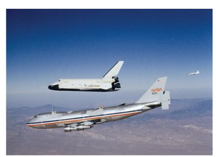
The Space Shuttle Enterprise was used to conduct approach and landing testing (1977) at the Dryden Flight Research Center, California. In the five free flights, the astronaut crew separated the spacecraft from the Shuttle Carrier Aircraft and maneuvered to a landing. These flights verified the Orbiter's pilot-guided approach and landing capability and verified the Orbiter's subsonic airworthiness in preparation for the first crewed orbital flight.
