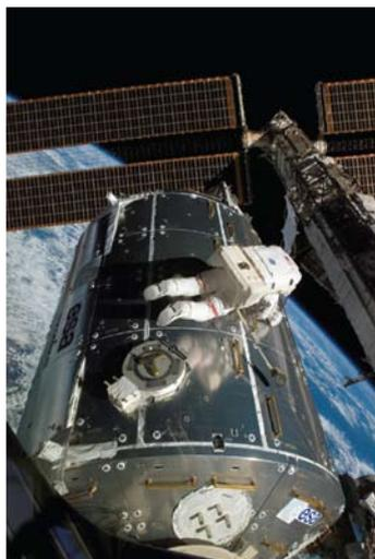
cubic meters) with 995 cubic feet (21.18 cubic meters) of habitable space and is permanently attached to the U.S. Harmony connecting module's starboard port.
