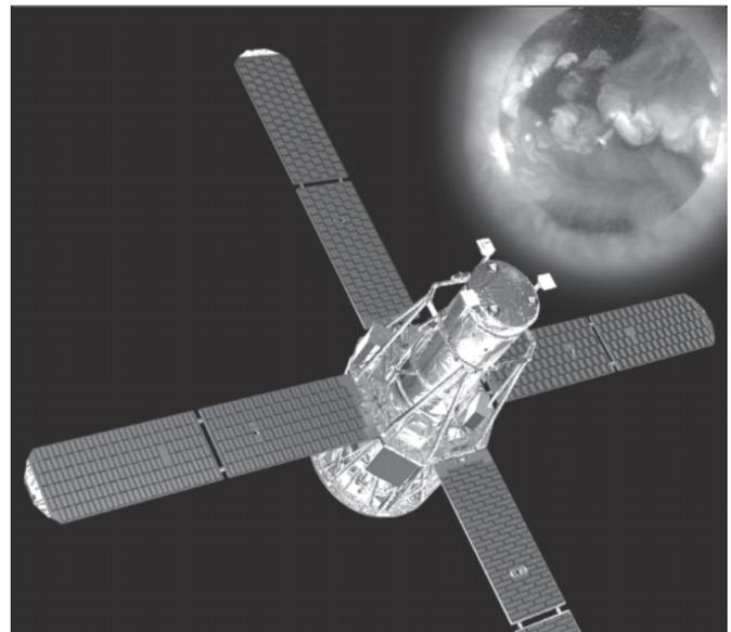
*Artist concept of the HESSI spacecraft studying solar flares from its circular orbit 373 miles (600 kilometers) above the Earth. (Image courtesy of Spectrum Astro, Inc.)*
