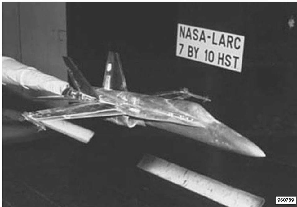
Figure 1. MD/Navy 6% F/A-18 model in the NASA Langley 7- × 10-ft High Speed Tunnel.
