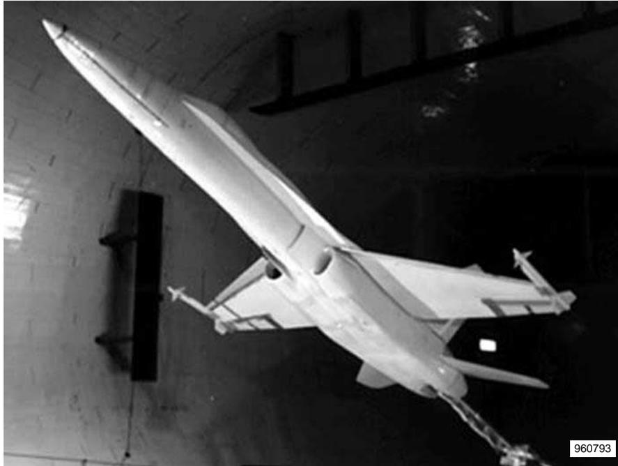
Figure 5. NASA-2 16% F/A-18 model in the NASA Langley 30- × 60-ft Tunnel.
