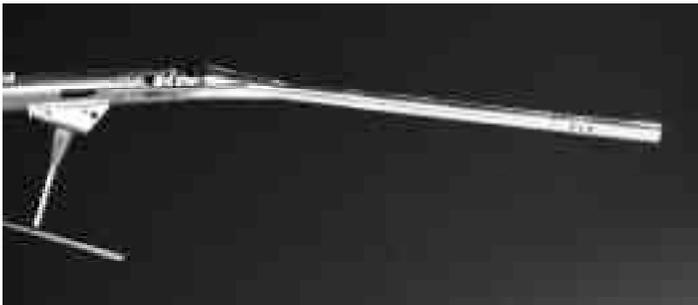
Side view of the Kiel probe on an X-31 showing the 10-degree bend downward. (NASA photo EC93-42024-1)
