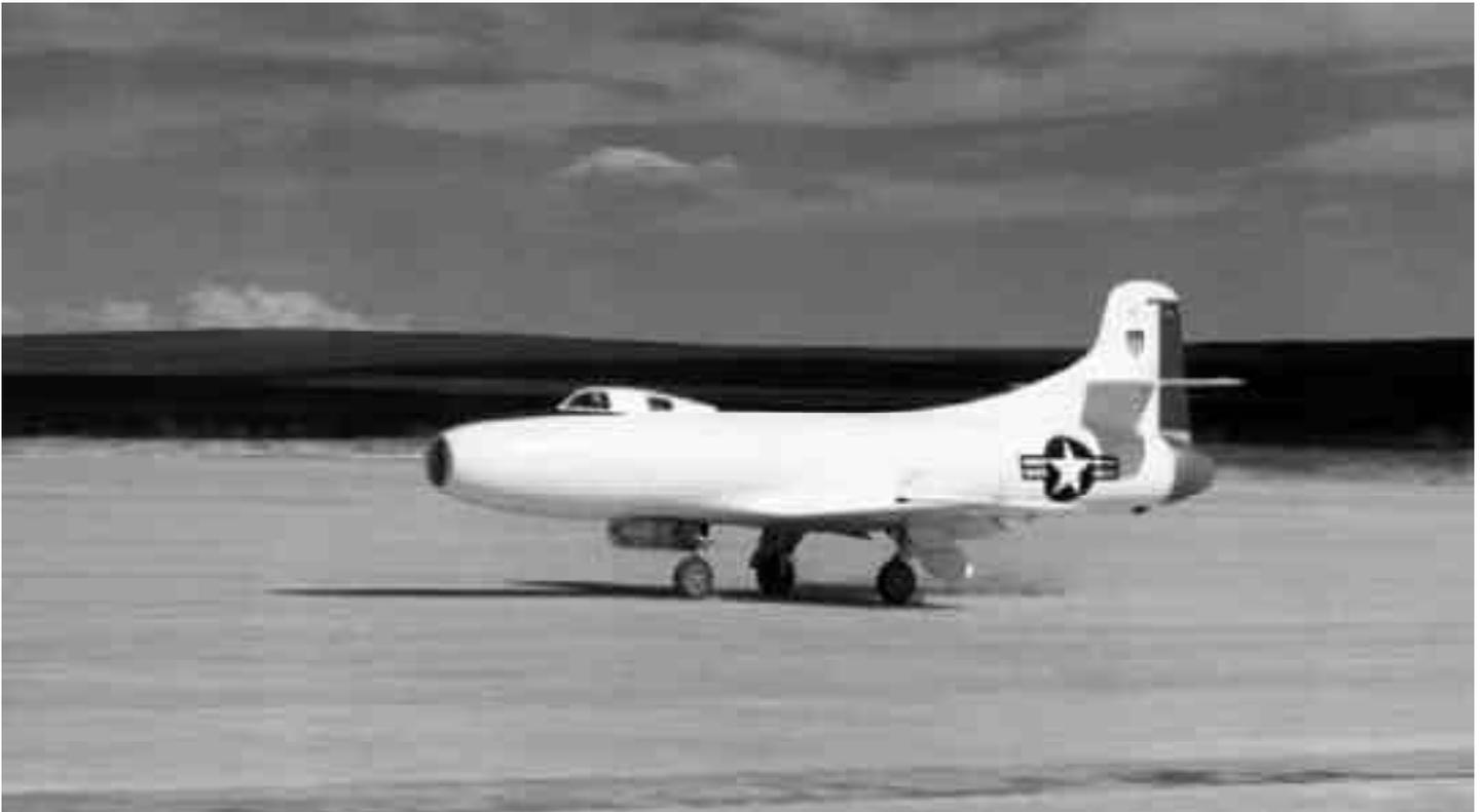
The D-558-I "Skystreaks" were among the early transonic research airplanes like the X-1, X-4, X-5, and XF-92A. Three of the single-seat, straight-wing aircraft flew in a joint program involving the National Advisory Committee for Aeronautics (NACA), the Navy-Marine Corps, and the Douglas Aircraft Co. from 1947 to 1953. In the process, the Skystreaks set several world speed records.
